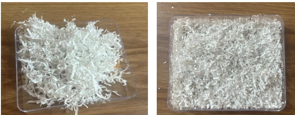
Figure 1. Visuals of waste PVC shavings used in the study
